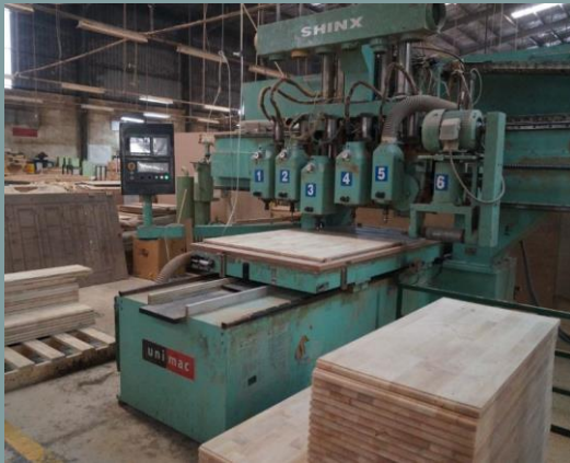
Router CNC – multiple drilling based on computer programed
