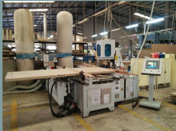
CNC multiple function of door process controlled by computer
