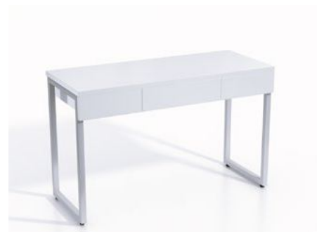
BLV002-ID3 97.25 USD R : 1200 x S : 600 x C : 750 The top is made from moisture resistant MDF, Glue E1, covered with anti-bacterial Laminate of Japan Aica. The drawer is made from MFC with the same color as Laminate. The edge is banded with ABS. The leg is SUS304
